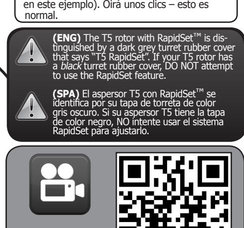
**(ENG)** The T5 rotor with RapidSet™ is distinguished by a dark grey turret rubber cover that says "T5 RapidSet". If your T5 rotor has a **black** turret rubber cover, DO NOT attempt to use the RapidSet feature.
