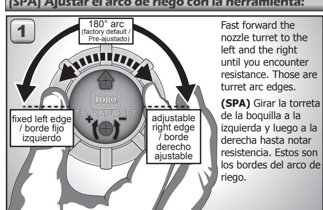
Fast forward the nozzle turret to the left and the right until you encounter resistance. Those are turret arc edges.
